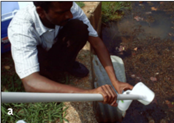
Figure G.1: A dipper (a) is helpful when the outfall is hard to reach. A milk jug (b) can be used to collect samples from shallow flow.
