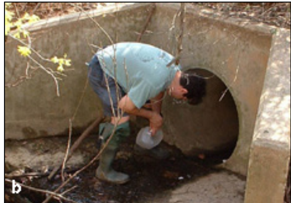
Figure G.1: A dipper (a) is helpful when the outfall is hard to reach. A milk jug (b) can be used to collect samples from shallow flow.
